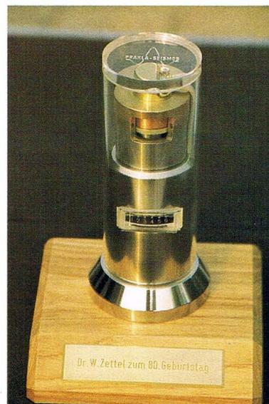
**The gift from the Technical Department: a 'geophone' with an indicator for sensing ground movement, an elaborate modification of the geophone which Dr. W. Zettel together with Dr. Friedrich Trappe registered for a patent in 1936. (Made by S. v. Jezierski)**
