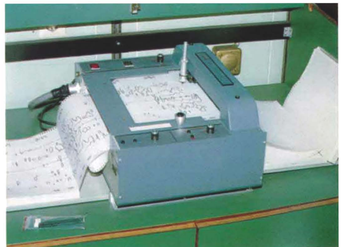
Fig. 4 On-line-Streifenplotter des Sea-Beam-Systems On-line strip plotter of the Sea Beam system
