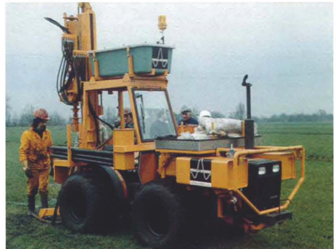
Impact hammer units for performing the newer displacement drilling technique with: pneumatic drive rotary drilling rig P 0501 (above), with hydraulic drive P 0152 (above right), and with mechanical drive ramhammer RH 130 S Pionjär (right)
