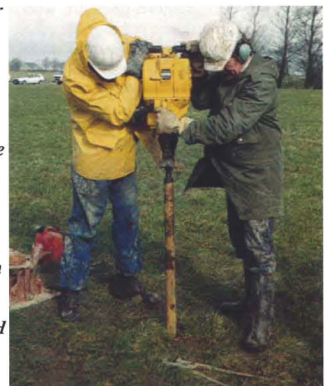
Impact hammer units for performing the newer displacement drilling technique with: pneumatic drive rotary drilling rig P 0501 (above), with hydraulic drive P 0152 (above right), and with mechanical drive ramhammer RH 130 S Pionjär (right)
